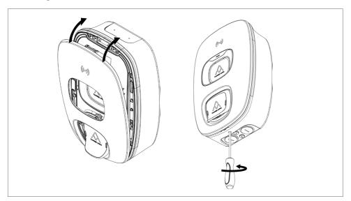
N.B. The front cover lock screw should not be removed. Use a max. torque of 2 Nm when tightening the screw
